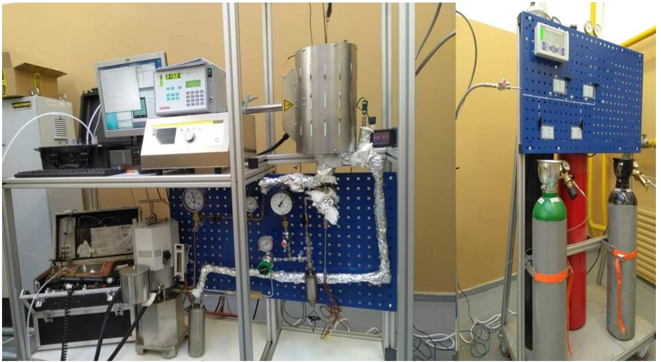
Figure 9. The laboratory experimental set up for CO 2 methanation
