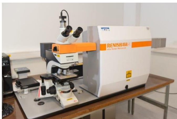
13 pav. Raman'o sklaidos spektrometras (Renishaw in Via, Wotton-under-Edge, UK)
