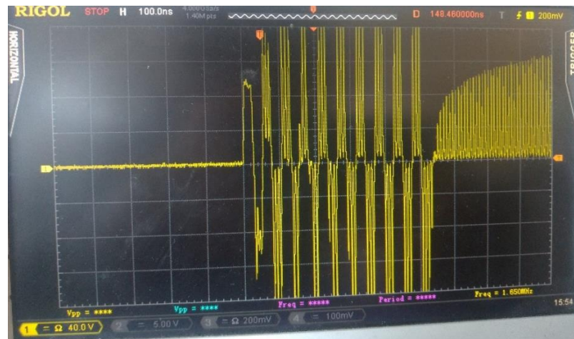
Fig. 5.2. Oscillations occurring on the output of the pulser (20 MHz, 100 V, 470 pF load)
