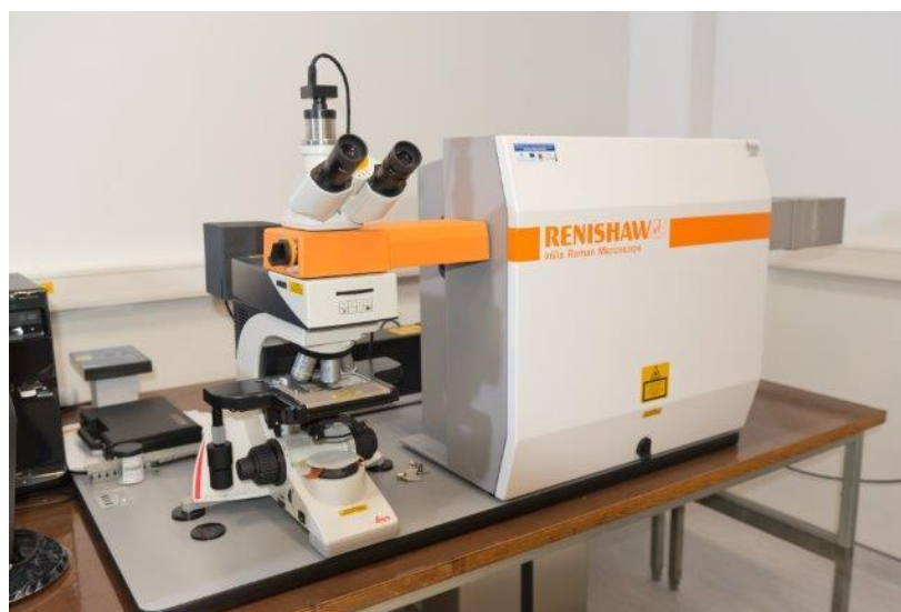
Fig. 26. The Raman spectroscopy photo (Renishaw in Via Spectrometer with accessories) used in National innovation and entrepreneurship center in KTU.
