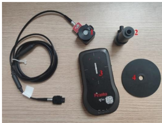
Figure 12. Equipment used for quantitative monitor measurements. Number 1 in the picture presents a cap for ambient light measurements, number 2 indicates a cap for luminescence measurements, number 3 is a device itself that processes the data and sends it to the computer, and number 4 is an extra detail for luminance measuring cap to make measurements more accurate by making them more directional.
