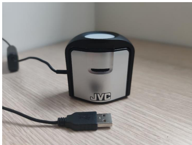
Figure 15. X-Rite i1Display Pro calibration device. It has an integrated photometer, colorimeter and is capable of measuring ambient light intensity.
