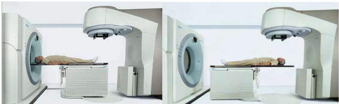
Fig. 9. Siemen's CTVision consisting of a Primus linear accelerator and a modified SOMOTOM diagnostic CT scanner [46]
