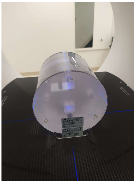
Fig. 24. Aligning of QUART phantom using laser on Halcyon system
