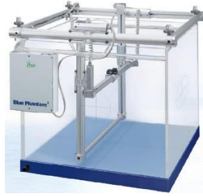
Fig. 9. Water phantom for absorbed dose measurement [81]
