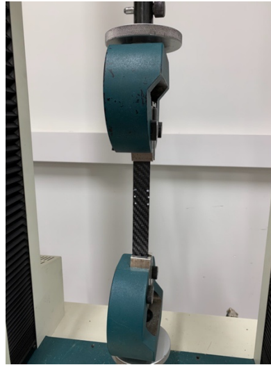
Fig. 21. Experimental set-up for CFRP tensile testing
