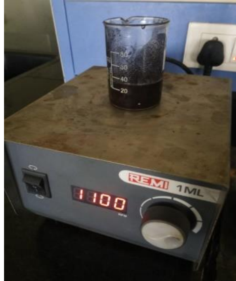
FIG. 41. Magnetic stirring of the MRF
