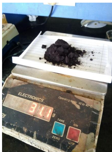
FIG. 37. Synthesized and weighted nickel iron oxide
