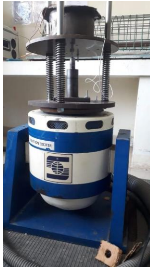
FIG. 44. Damper mounted on the Quarter car model in the vibration shaker
