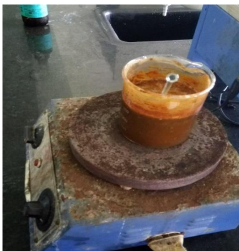
FIG. 32. Heating the nickel carbonate and ferric chloride solution
