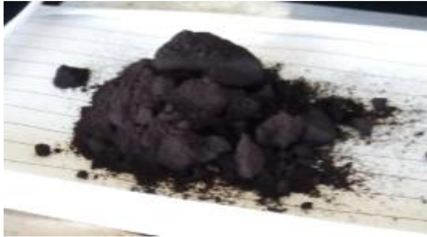
FIG. 25. Nano particles of nickel iron oxide
