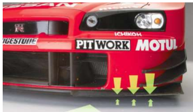
Fig. 5. Airflow by the Splitter [9]
