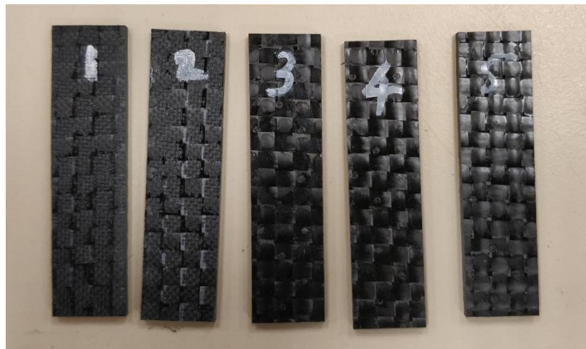
Fig. 30. Short beam test specimens
