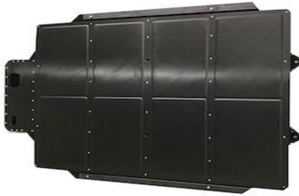
Fig. 4. SGL Carbon's - Carbon fibre-based battery enclosure for NIO electric vehicles [5].
