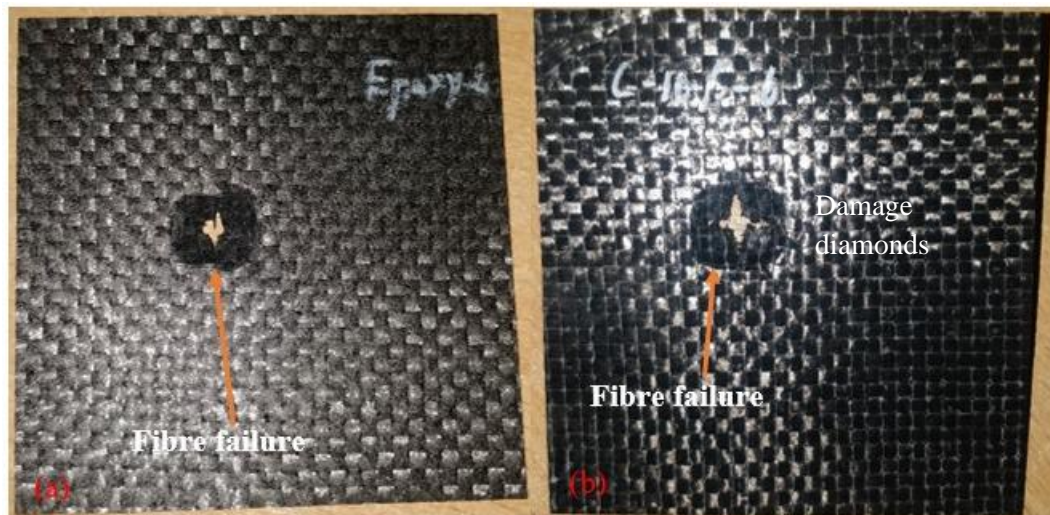
Fig. 42. Specimens with fibre failure (a) pure epoxy composite (b) Ace MX-960 at 10 wt.% modified composite
