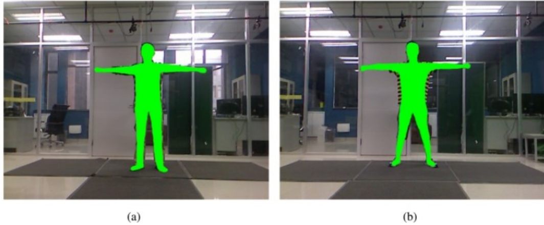
Fig. 2. Results for the reduction of the clothes effect: (a) a person wearing tight clothes; (b) a person wearing loose clothes [15]
