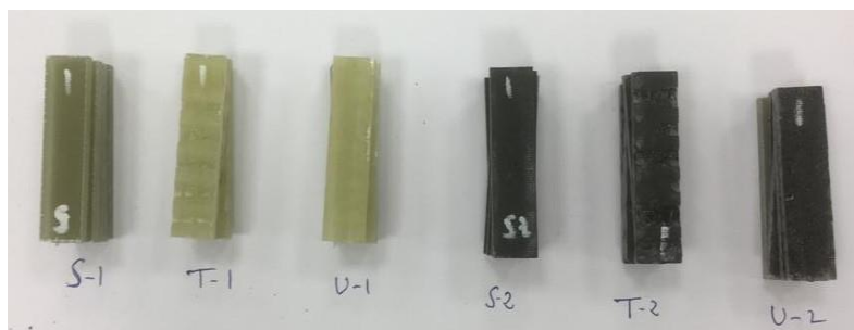
Fig. 16. Specimens for interlaminar shear test
