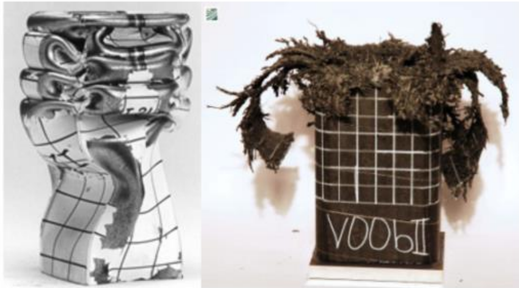
Fig. 3. Behaviour of metal and FRP under impact[2].
