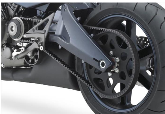
1.8 pav. Mid-drive pavaros tipas [12].
