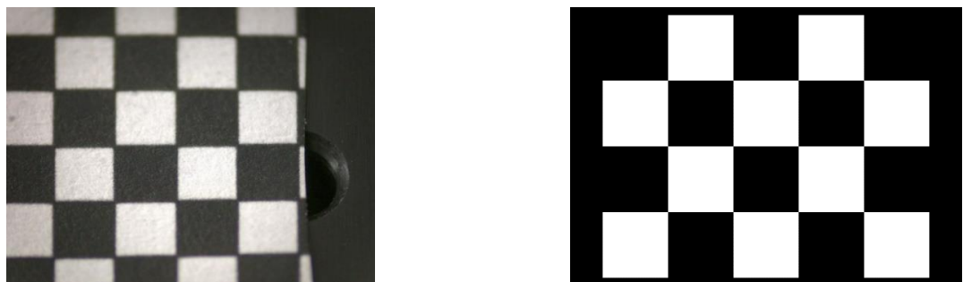
Fig. 56. Checkerboard pattern viewed by the microscopic lens (left) vs an ideal checkerboard pattern for accurate calibration (right)
