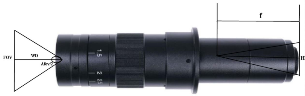
Fig. 50. Focal length and working distance relationship [30]
