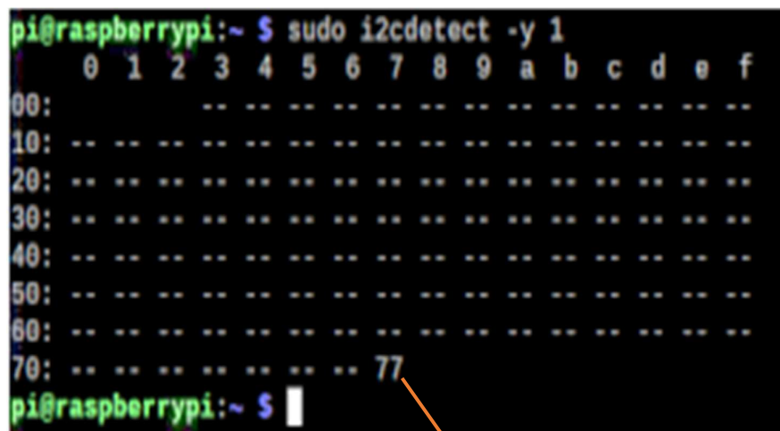
Fig. 27. Connection of BMP180 sensor with raspberry pi
