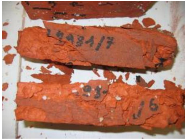
Fig. 12. Defects appeared during the freeze and thaw test [27]
