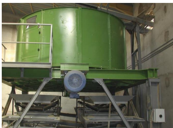
Fig. 38. Modern clay mixing and weighting hopper [33]
