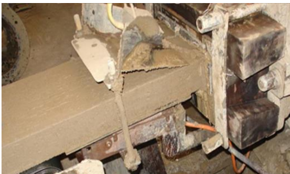
Fig. 24. Extruded bar of clay S3
