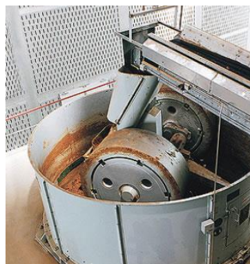
Fig. 22. Clay mass mixing process
