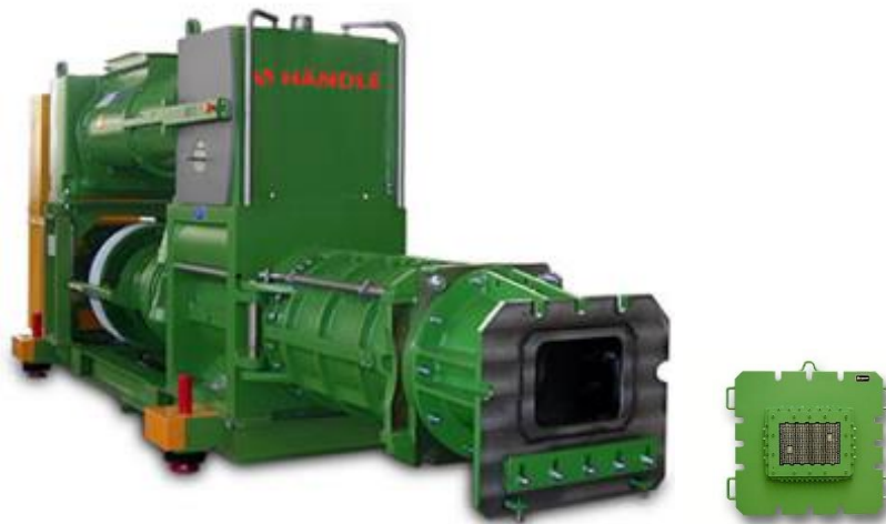
Fig. 23. Clay shaping machine [31]
