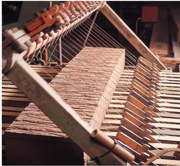
Fig. 26. Clay bar cutting machine [7]
