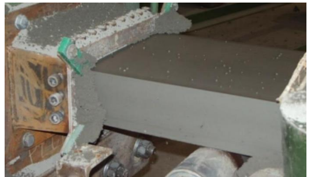
Fig. 25. Extruded bar of clay S2
