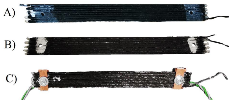
Fig. 37. Specimen’s preparation procedure for three-point bending experiment: a) polished specimen with drilled holes; b) specimen with silver paint applied around holes; c) electrodes and copper plates attached to the specimen
