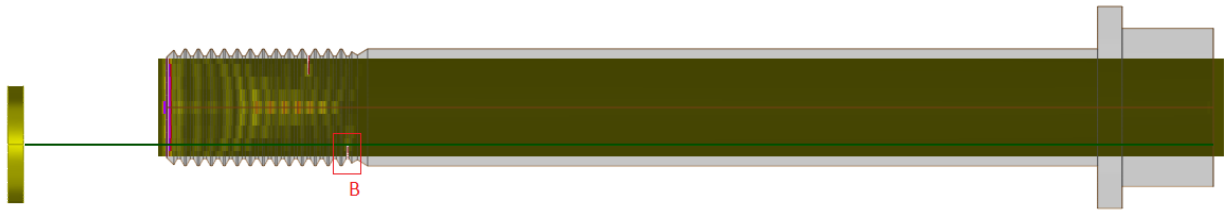
Figure 2-8. 3D scan view, defect at the incomplete thread root area and placed notch (B)
