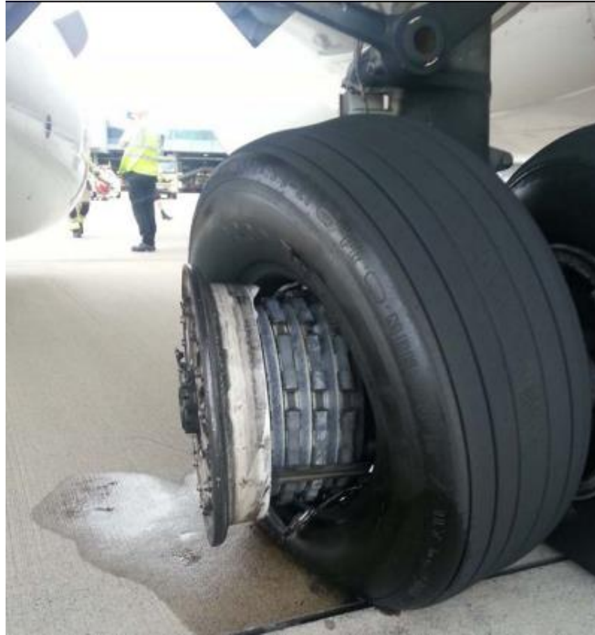
Figure 1-2. Damage to the number one main wheel assembly on VUH [5]
