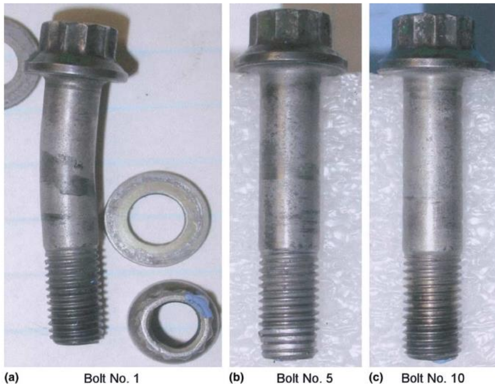
Figure 1-3. Photographs of bolts from each damage category: (a) bent; (b) stripped (note last four threads of Bolt #5), and (c) no apparent damage [6]
