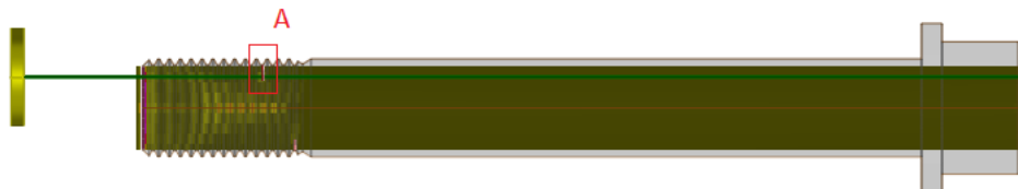
Figure 2-5. 3D Scan right view, defect at the third complete root area and placed notch (A)
