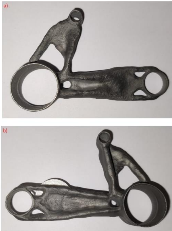
Fig. 2.29. Manufactured part; a) upskin, with visible layer lines; b) downskin with visible support area
