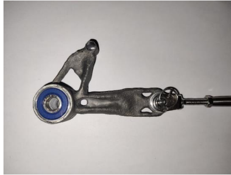
Fig. 2.33. Completed part with bearings and tension rod
