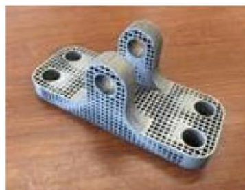
Fig. 1.18. Variable density lattice infill [36]
