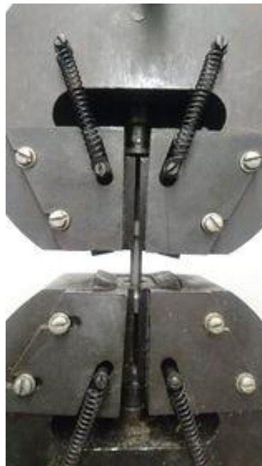
Fig. 2.8. Specimen fitted in the 2054 P-5 testing machine
