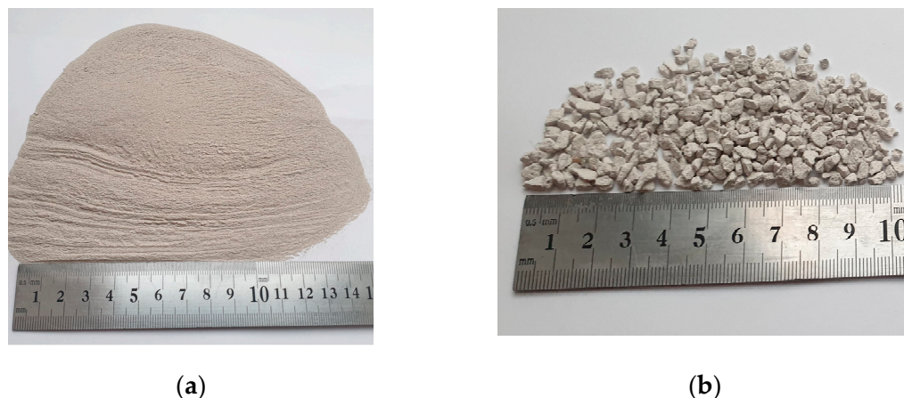
Figure 7. Photograph of the: (a) zeolitic by-product; (b) coarser fraction of sorption material based on straetlingite.
