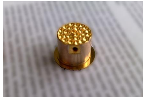
Figure 8. Ultrasonic transducer with a graphite bronze backing on the top.
