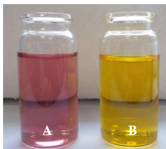
Fig. 3.2. Collected BnF (A) and VxF (B) fractions after separation of beetroot juice by HPLC system
