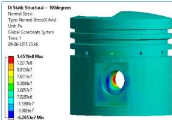
Fig 5.38 Al 413.0 Normal stress without combustion pressure @ 100°C
