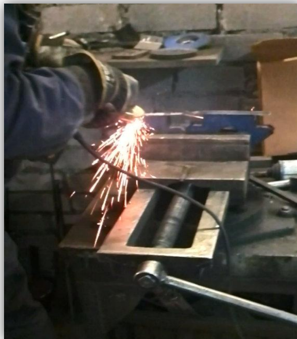
Fig. 2.15. Grinding process of a soiled glue wiper by using Bosch grinder
