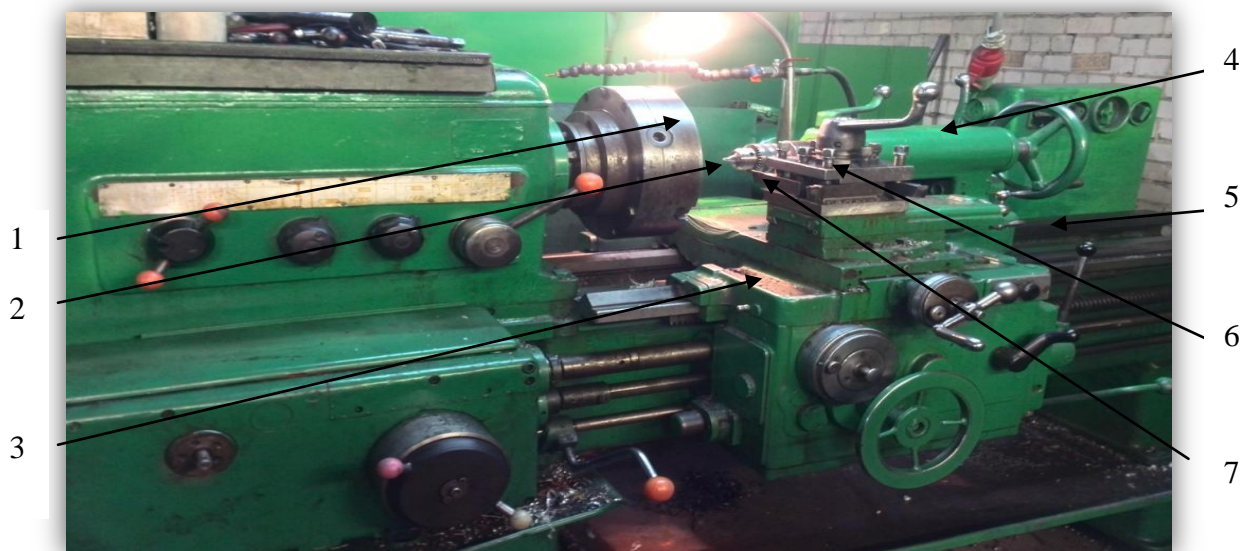
Fig.2.3. Engine lathe 16K20 and main its' parts
