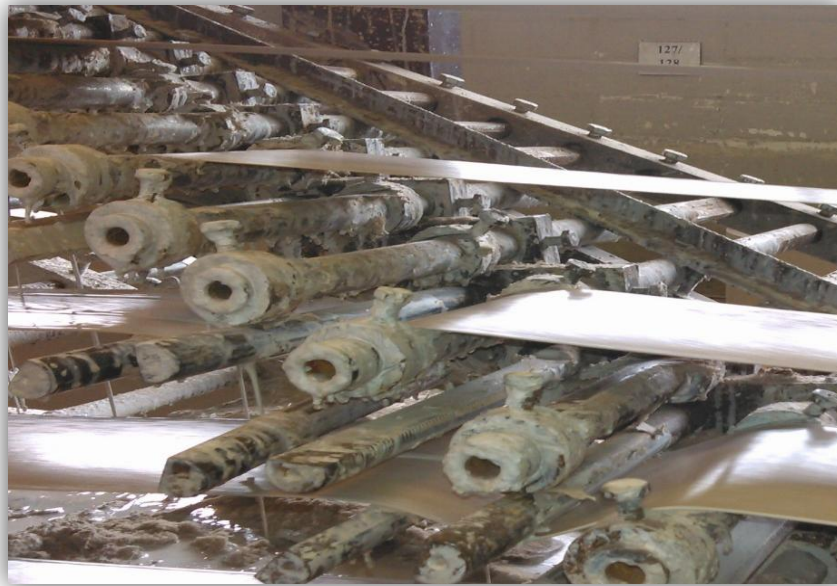
Fig.2.2. Soiled glue wipers after one week of glue cleaning
