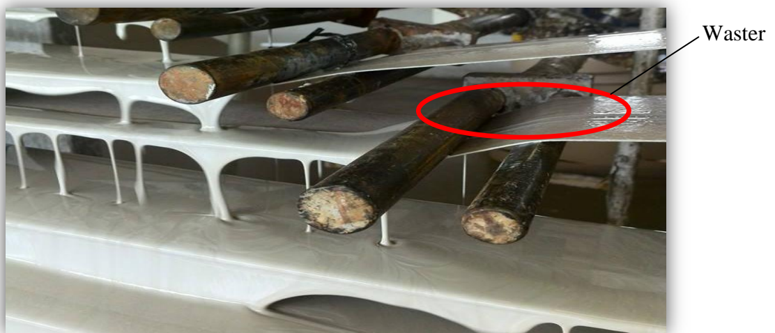
Fig.1.9. Waster of worn-out glue wiper
