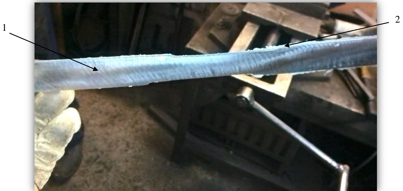
Fig. 2.16. Cleaned glue wiper after using Bosch grinder
