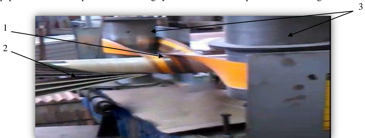
Fig.1.4. Winding mechanism in the standard cardboard tubes production line
