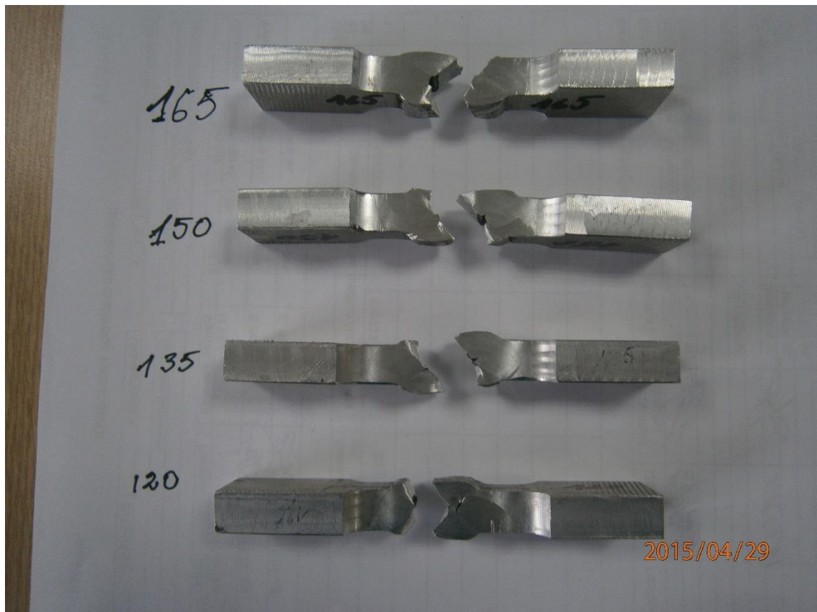
Fig3.3.6 welded specimens on after tensile testing procedure.
