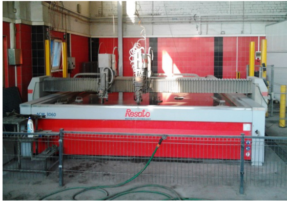
Fig. 2 The AWJ cutting machine ACM 3060-2
