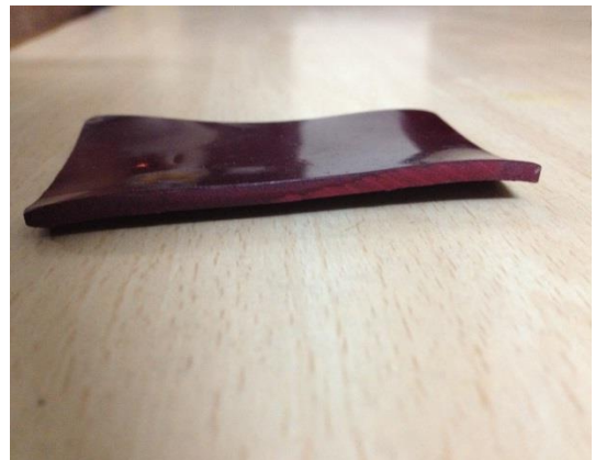
Figure 4.7 Part of motor cover after testing
