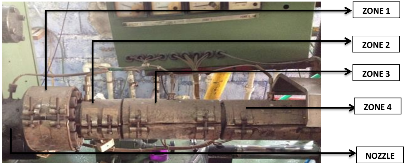
Figure 3.2 Barrel of injection molding machine
