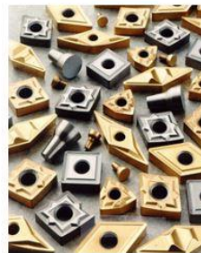
Figure 3.3: Different types of cemented carbide inserts for use by different cutting tools [19]
