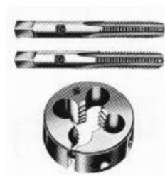
Figure 3.1: Thread tap and die made of high-speed steel [19]
