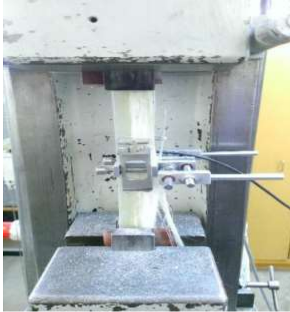
Figure 2.5: Tensile test specimen during the test
