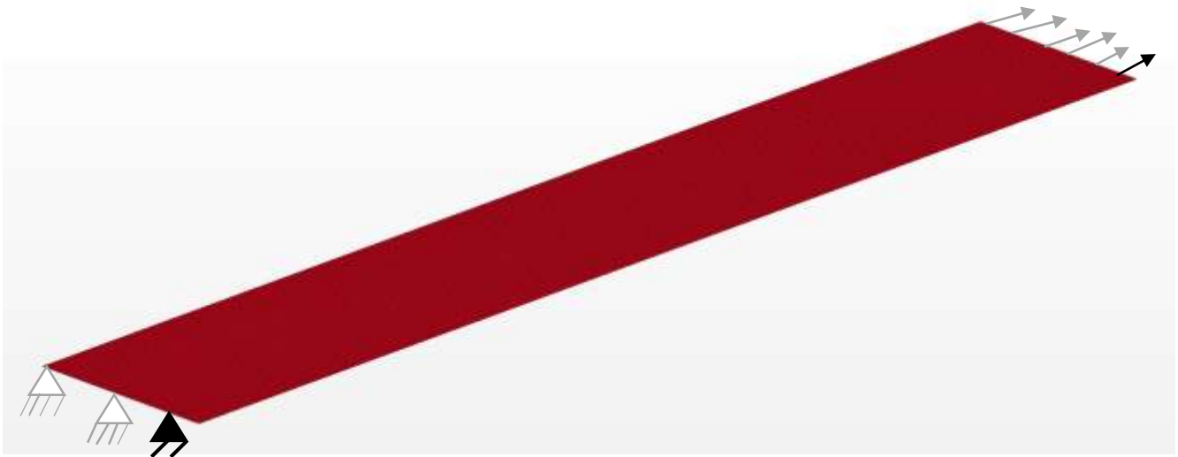
Figure 4.4: GFRP laminate with fixed nodes and loads applied nodes
