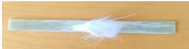
Figure 2.6: Tensile test specimen after the test (30°)
