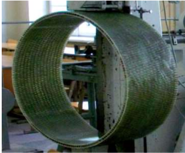
Figure 2.8: Experimental testing on GFRP Cylinder Ring
