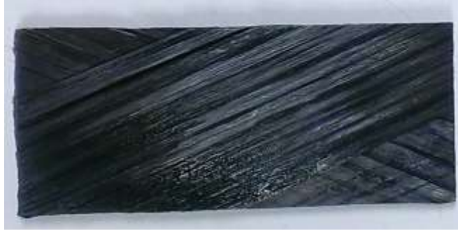
Figure 3.3: The angle of ply in GFRP laminate
