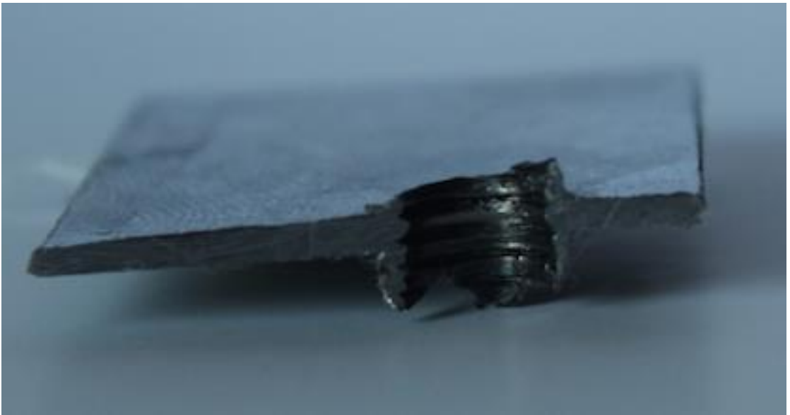
Figure 5.11: Cross-sectional view of S235JR Steel after tightening
