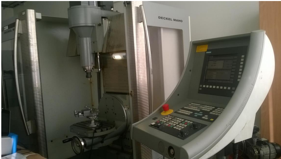
Figure 5.2: CNC Milling machine used for our experiment (DECKEL MAHO)
