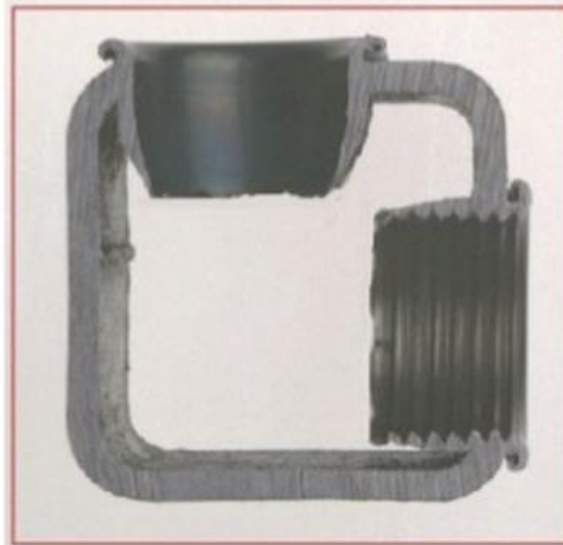
Figure1.2 Cross-section of hole and brushing [4]
