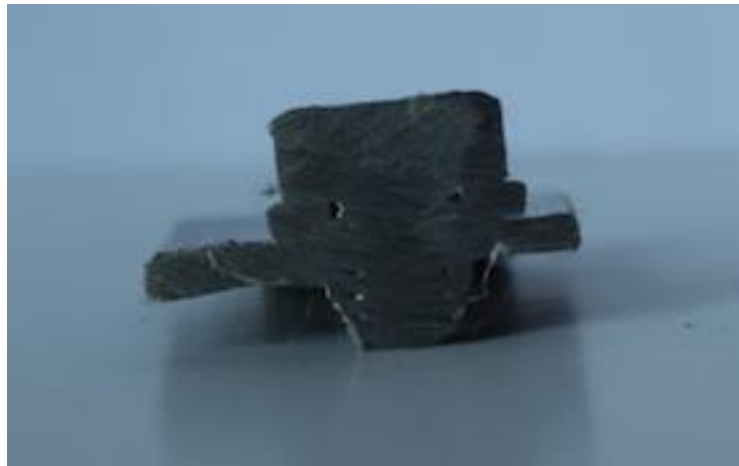
Figure 5.8: Cross-sectional view of Titanium plate with bolt
