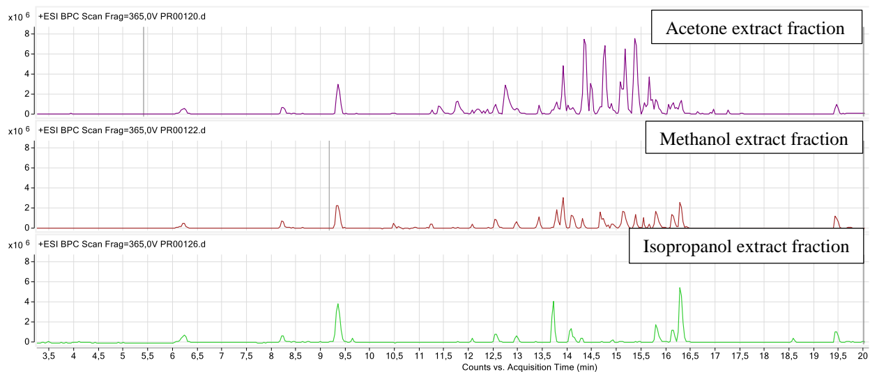
Figure 21. Base peak chromatograms of three biomass crude extracts.
