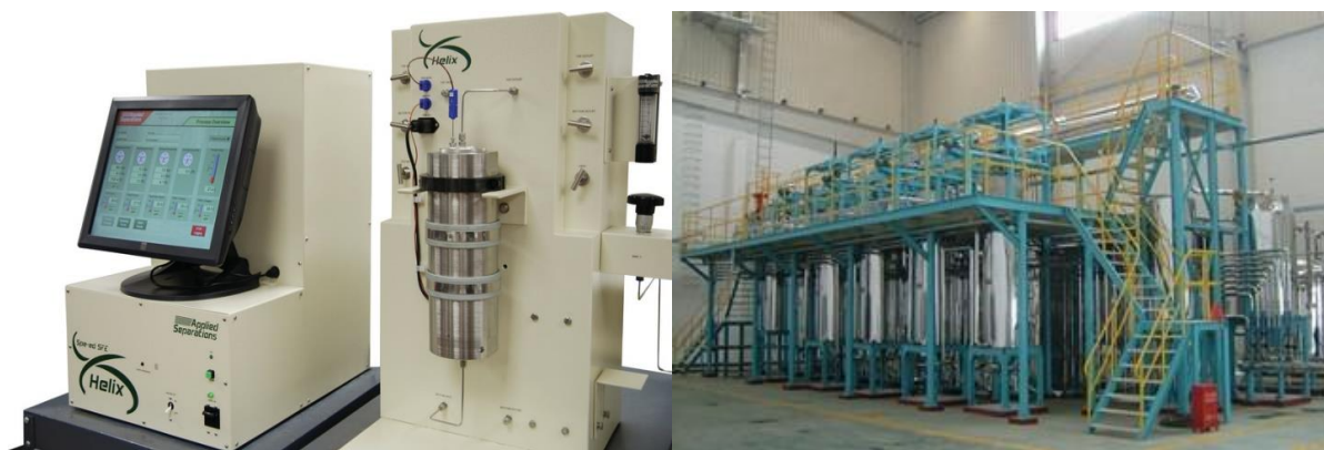
Figure 8. Laboratory (left) and industrial (right) supercritical fluid extractors.
