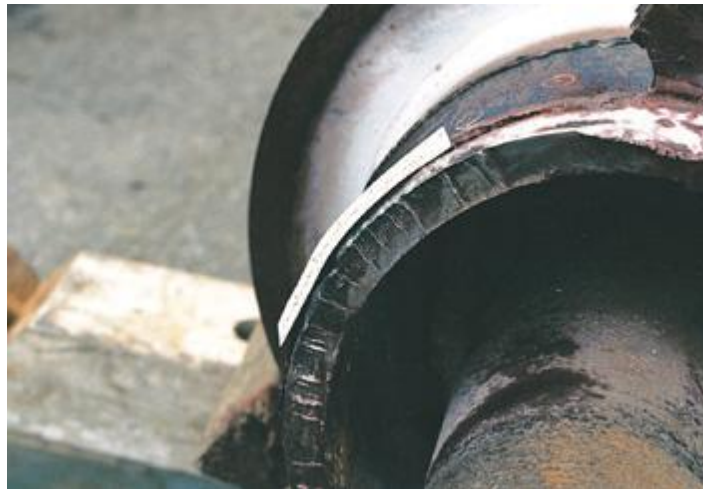
Figure 1.4 Shows the excessive loads conditions frequently result in fatigue failures in the shaft, reference [9]
