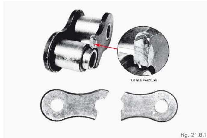
Fig.3.2 Fatigue fracture in link [37]
