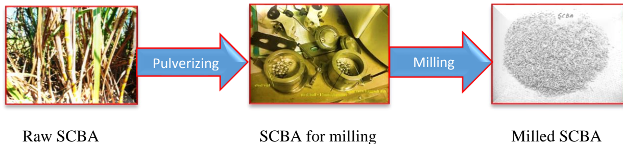
Figure - 8 Sugarcane Baggase Ash Processing
