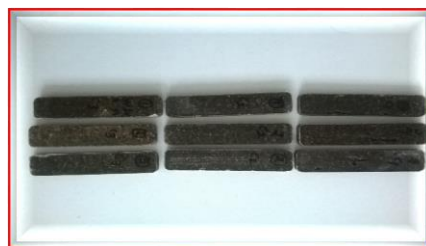
Specimen of 40% reinforcement (Natural plant fiber) and 60% Matrix (Vinyl Ester)
