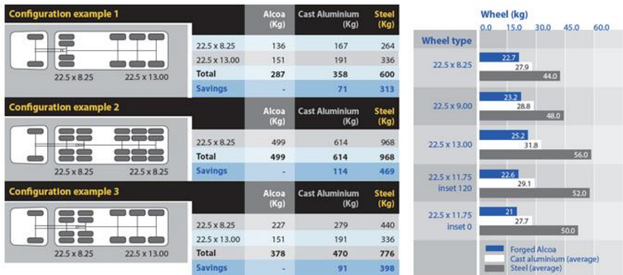
1.2.2. Picture: The weight difference between an Alcoa and a steel wheel [4]
