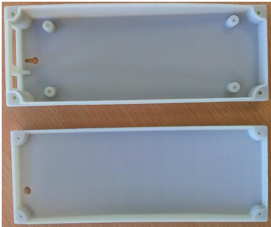
Fig. 3.9 Washed out model without support material
