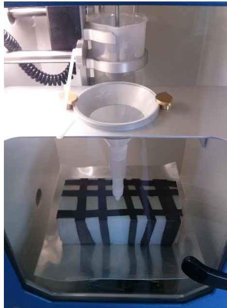
Fig. 3.23 Cast under vacuum in silicone mold
