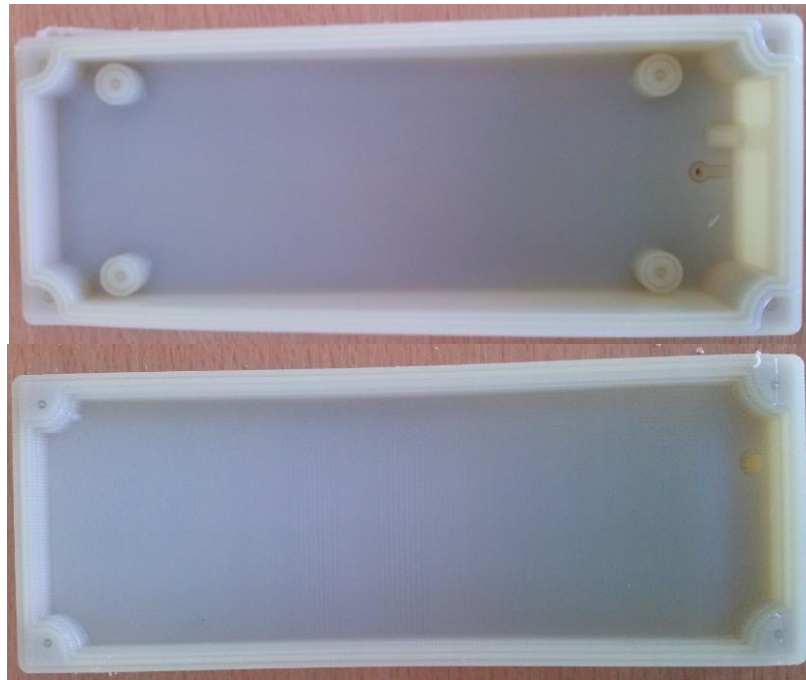
Fig. 3.8 Printed model: Shown above - bottom part, b) Shown below - top part
