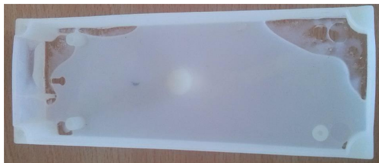
Fig. 3.24 Poorly casted detail
