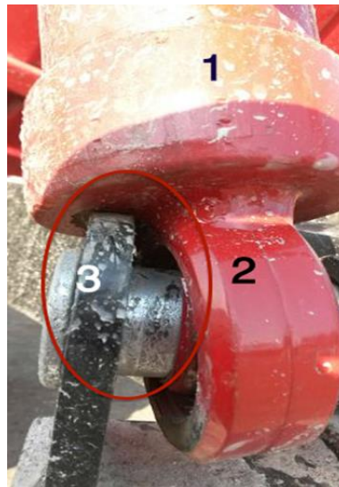
Fig. 3.22 Cylinder retainer node 1. Support, 2. Cylinder pin 3. Cylinder
