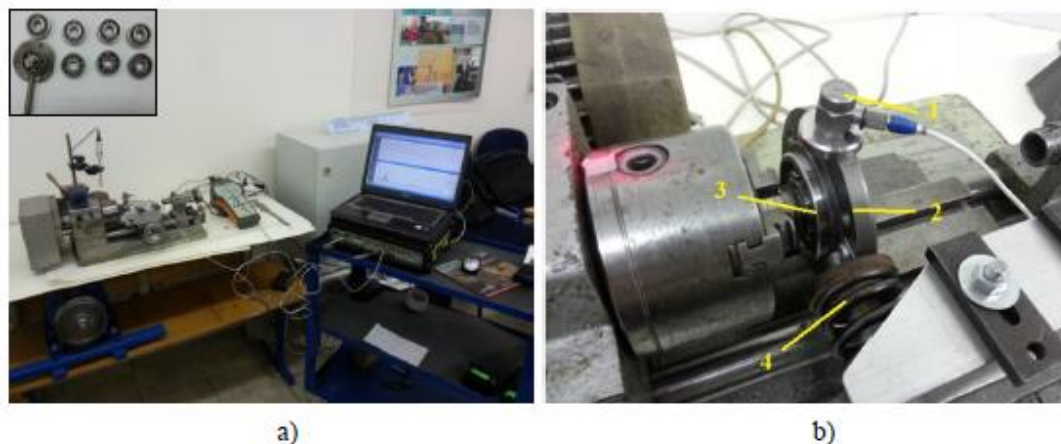
Figure 2. The experimental stand with the damaged 6303 type bearings (a); the radial load being applied to the bearing mount (b): 1 – accelerometer; 2 – bearing mount; 3 – bearing; 4 – compression spring.
