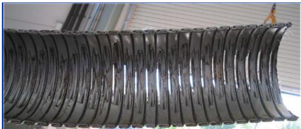
Fig – 3 Cross section view of carcass layer [53]
