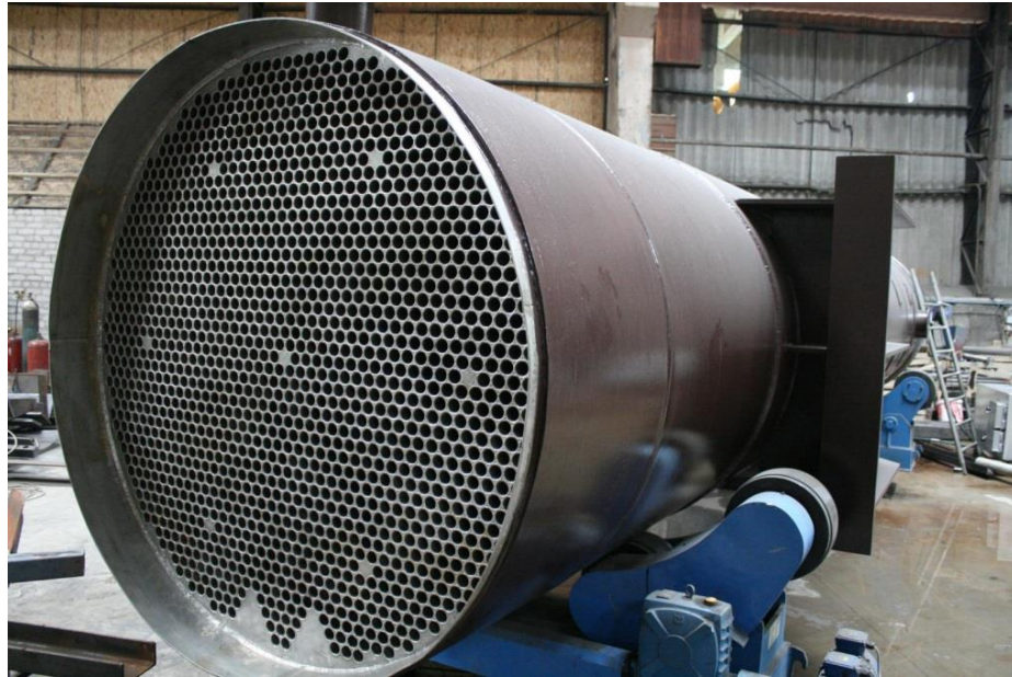
Fig. 13 Example of condensing economizer inner construction
