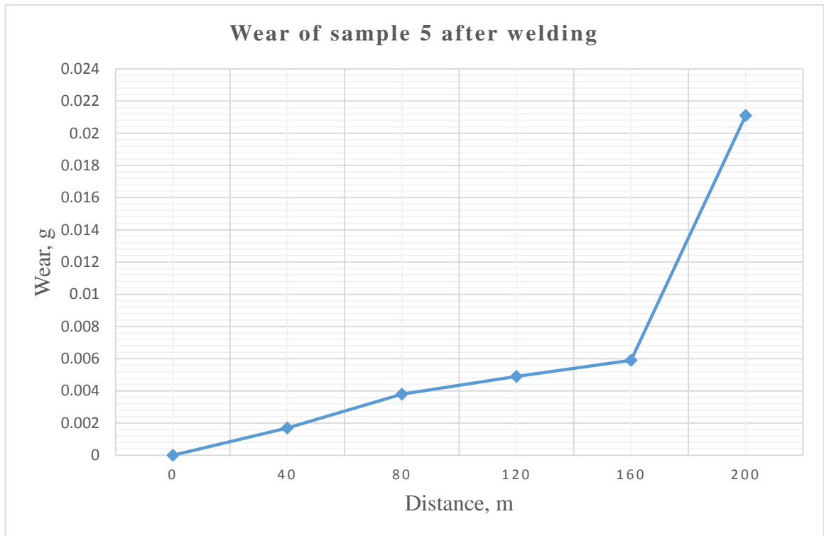
Figure 3.23 Wear of sample 5 after welding
