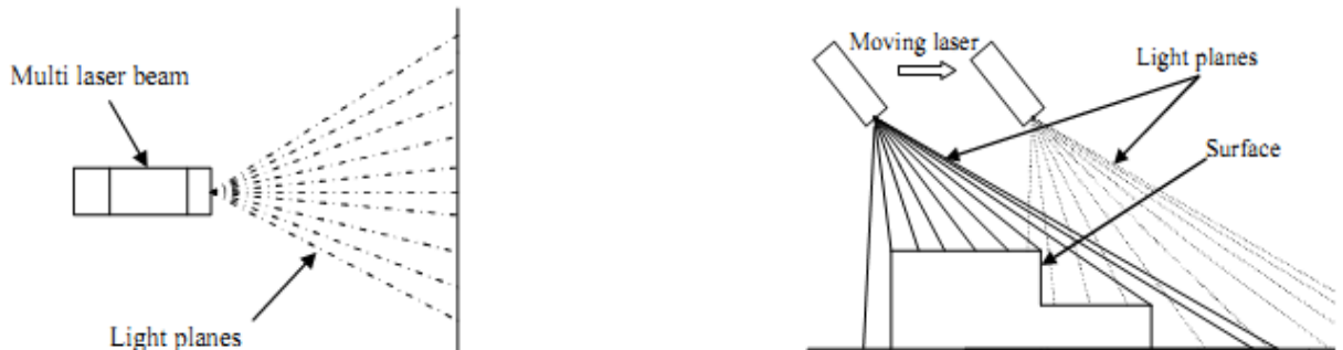
Fig. 3-10 Illustration of a multi beam laser and the emitted sheets of light and its area of coverage
