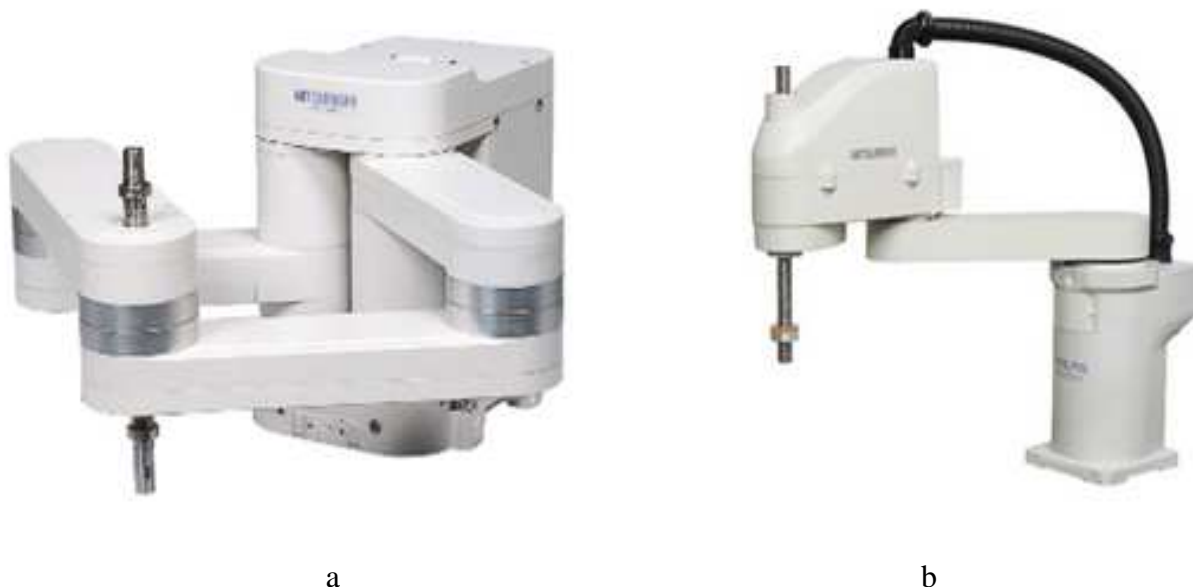
1 pav. Mitsubishi Electric robotai [2]: a – paralelinis, b - linijinis
