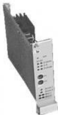
Fig. 3.11 Frequency generator HG 57500 [22]
