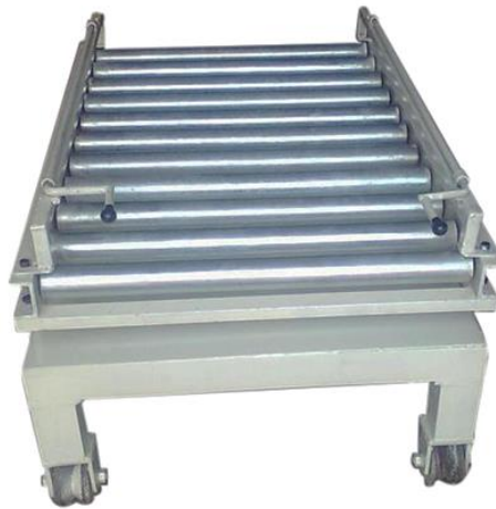
Fig. 2.5 Roller conveyer for the easier robot loading [10]
