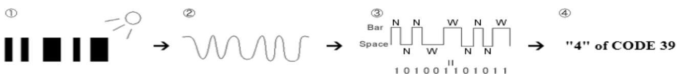
Fig. 3.4 Principle of bar code reading [15]
