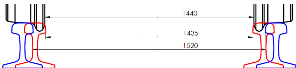
Fig. 2.5. Symmetrical layout, wider gauge wheel-set, P50 profile rails
