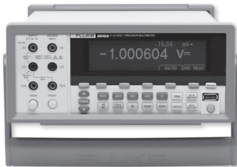
3.5 pav. Fluke 8846A skaitmeninis multimetras [13]
