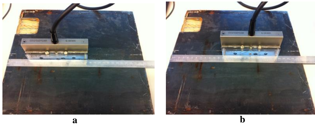
Fig.4.7. Experimental set-ups of defect evaluation in joint of steel and GFRP: a-inspection of 1st and 2nd delaminations, b- inspection of 2nd and 1st delaminations
