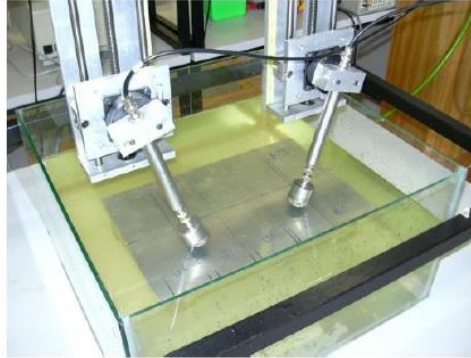
Fig.1.5. Experimental set-up of Lamb wave testing of adhesively bonded joints [11]
