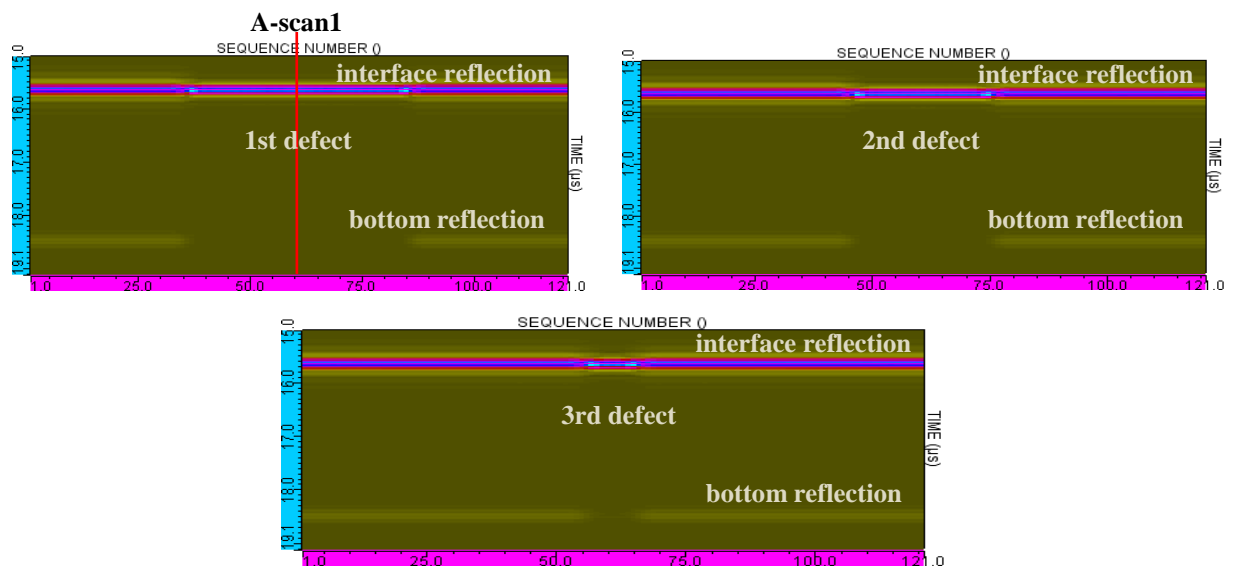
Fig.3.31. B-scans of the inspection from the metal side with 10 MHz phased array transducer
