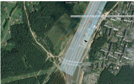
Fig. 3. Aerial imaging of bypass: flight strips numbered from 1 to 7
