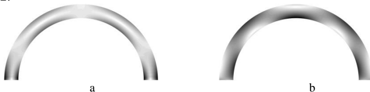
Fig. 22. Equivalent stresses the first eigenmode (a), the fourth eigenmode (b)
