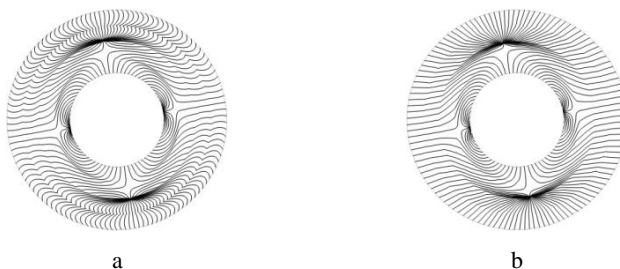
Fig. 20. Composite isoclinic patterns for second eigenmode obtained by using the procedure of conjugate approximation (a) and by using the proposed procedure of conjugate smoothing (b)
